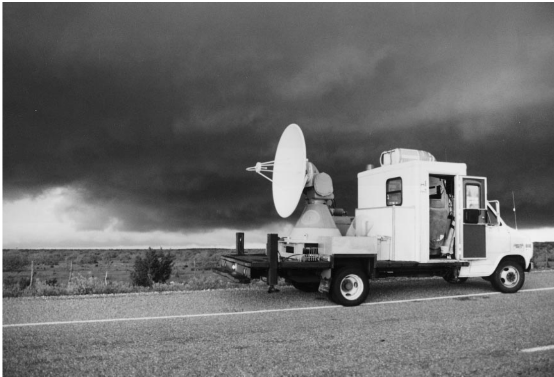
FIG. 4. The DOW scanning threatening weather during the VORTEX-95 field program. The 6' dish and operator cabin are visible.
