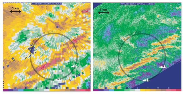
FIG. 4. Radar reflectivity (dBZ) observations of a narrow cold-frontal rainband at 0351 UTC 3 Nov 2004 as seen by the (left) KCCX WSR-88D and (right) DOW2. The DOW2 reflectivity is uncalibrated. The locations of the two DOW radars and the dual-Doppler lobe are overlaid.
