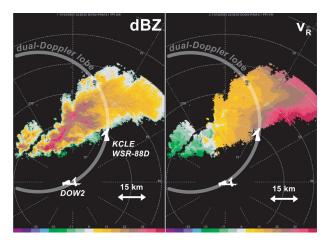
FIG. 2. (left) Reflectivity (dBZ) and (right) radial velocity (m s<sup>-1</sup>) observations by DOW2 of a severely sheared, low-topped thunderstorm near Cleveland, Ohio, at 2331 UTC 12 Nov 2003. The environment was characterized by exceptionally strong vertical wind shear (0–6 km shear of ~50 m s<sup>-1</sup>). The DOW2 reflectivity is uncalibrated. The locations of the KCLE WSR-88D and dual-Doppler lobe are overlaid.
