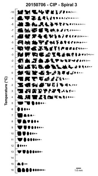
Fig. 6. Representative particles imaged by the 2DC probe during the spiral descent of the NOAA P-3 through the trailing stratiform region between 0440 and 0453 UTC 6 Jul 2015. This flight section is shown in pink in Fig. 4.
