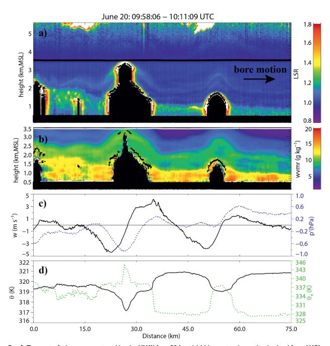
Fig. 9. Transect of a bore encountered by the UWKA on 20 Jun. (a) Lidar scattering ratio obtained from WCL above flight level (3.55 km MSL) and CRL below flight level; (b) CRL water vapor mixing ratio; (c),(d) flight-level data, including air vertical velocity w, perturbation pressure p, potential temperature  $\theta$ , and equivalent potential temperature  $\theta_e$ .
