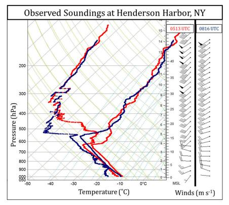
FIG. 4. Soundings launched at 0513 UTC (red) and 0816 UTC (blue) 7 Jan 2014 from Henderson Harbor. Horizontal winds (m s<sup>-1</sup>; half barb = 5, full barb = 10, and pennant =  $50 \text{ m s}^{-1}$ ) for both soundings are plotted along the right side of the image.
