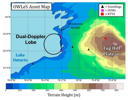
FIG. 1. OWLeS asset map from 7 Jan 2014. The DD lobe from DOW6 and DOW8 is drawn in black; the radar baseline is 16.4 km. The locations of DOW6 and DOW8 are marked with magenta dots (DOW8 to the north; DOW6 to the south), the Montague, NY, WSR-88D (KTYX) location is marked with a red square, and the mobile sounding locations are marked with black triangles.
