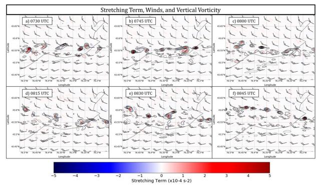
FIG. 27. Stretching term (×10<sup>-4</sup> s<sup>-2</sup>; shaded) from the WRF simulation (333-m domain) at 500 m AGL. Horizontal winds (m s<sup>-1</sup>; half barb = 5 and full barb = 10 m s<sup>-1</sup>) and relative vertical vorticity (contoured every  $0.5 \times 10^{-2} s^{-1}$  starting at  $-5.5 \times 10^{-2} s^{-1}$ ; solid = positive and dashed = negative) valid at (a) 0730, (b) 0745, (c) 0800, (d) 0815, (e) 0830, and (f) 0845 UTC 7 Jan 2014.
