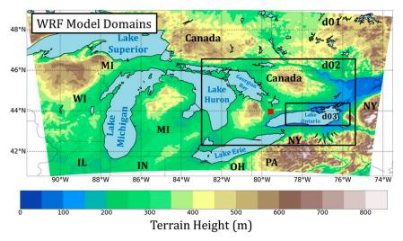
FIG. 2. Domains of the WRF Model simulation. The outermost domain (d01; 1335 km  $\times$  882 km) has a horizontal grid spacing of 3 km, the middle domain (d02; 636 km  $\times$  438 km) has a horizontal grid spacing of 1 km, while the innermost domain (d03; 258 km  $\times$  147 km) has a horizontal grid spacing of 333 m. Terrain height is plotted in meters (shaded). The King City, Ontario (CWKR), radar location is marked with a red square.
