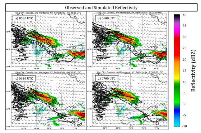
FIG. 18. Composite reflectivity (dBZ; 10- and 15-dBZ contours shown) and 500-m AGL horizontal winds (m s<sup>-1</sup>; half barb = 5 and full barb =  $10 \text{ m s}^{-1}$ ) from the WRF simulation (1-km domain) overlaid with KTYX and CWKR base reflectivity (dBZ; shaded) valid at (a) 0530, (b) 0600, (c) 0630, and (d) 0700 UTC 7 Jan 2014.
