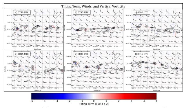
FIG. 26. Tilting term ( $\times 10^{-4}$  s<sup>-2</sup>; shaded) from the WRF simulation (333-m domain) at 500 m AGL. Horizontal winds (m s<sup>-1</sup>; half barb = 5 and full barb = 10 m s<sup>-1</sup>) and relative vertical vorticity (contoured every  $0.5 \times 10^{-2}$  s<sup>-1</sup> starting at  $-5.5 \times 10^{-2}$  s<sup>-1</sup>; solid = positive and dashed = negative) valid at (a) 0730, (b) 0745, (c) 0800, (d) 0815, (e) 0830, and (f) 0845 UTC 7 Jan 2014.
