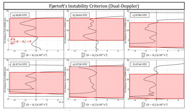
FIG. 14. The quantity  $(\partial^2 \overline{u}/\partial y^2)(\overline{u} - \overline{u}_l)$  (×10<sup>-6</sup> s<sup>-2</sup>) vs north–south distance (km) from DOW6 at 500 m AGL valid at (a) 0630, (b) 0644, (c) 0700, (d) 0714, (e) 0730, and (f) 0744 UTC 7 Jan 2014. The red shaded rectangles indicate where FIC is satisfied.
