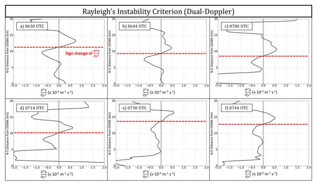
FIG. 13. The quantity  $\partial^2 \overline{u}/\partial y^2$  (×10<sup>-6</sup> m<sup>-1</sup> s<sup>-1</sup>) vs north–south distance (km) from DOW6 at 500 m AGL valid at (a) 0630, (b) 0644, (c) 0700, (d) 0714, (e) 0730, and (f) 0744 UTC 7 Jan 2014. The red dashed lines denote the locations where RIC is satisfied.
