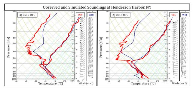
FIG. 17. Observed (red) and WRF-simulated (blue; 333-m domain) soundings at Henderson Harbor at (a) 0515 and (b) 0815 UTC 7 Jan 2014. Winds (m s<sup>-1</sup>; half barb = 5, full barb = 10, and pennant = 50 m s<sup>-1</sup>) for both soundings are plotted along the right side of each image.
