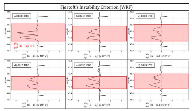
FIG. 25. The quantity  $(\partial^2 \overline{u}/\partial y^2)(\overline{u} - \overline{u}_I) (\times 10^{-6} \text{ s}^{-2})$  vs latitude (°) from the WRF simulation (333-m grid) at 500 m AGL valid at (a) 0730, (b) 0745, (c) 0800, (d) 0815, (e) 0830, and (f) 0845 UTC 7 Jan 2014. The red shaded rectangles indicate where FIC is satisfied.
