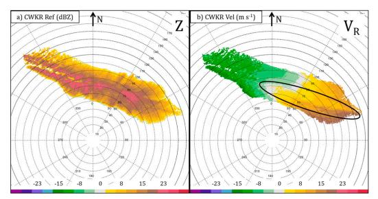
FIG. 11. The  $0.2^{\circ}$  CWKR (red square in Fig. 2) (a) reflectivity (dBZ) and (b) radial velocity (m s<sup>-1</sup>) at 0523:35 UTC 7 Jan 2014. Range rings are plotted every 10 km and azimuth angles are plotted every 30°. The black oval denotes the location of the cyclonic horizontal shear zone discussed in the text.
