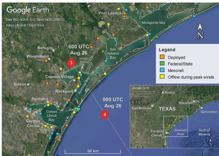
FIG. 1. Map of all in situ and adaptive surface assets deployed for Hurricane Harvey. Yellow labels indicate stations that did not capture peak winds due to, for example, station failure/destruction, loss of power, loss of connectivity, or loss of data. The dataset was significantly enriched by the private mesonet assets, most notably in the swath of very high impact from Holiday Beach, through Rockport, and to Port Aransas. The more specialized adaptive and local mesonet observations proved to be collectively more reliable than the in situ state and federal networks, yielding a 74% success rate in capturing peak winds over land vs only 36% for the state and federal sites. Indeed, only 5 federal/state stations (shown in green) out of 14 were online when the peak winds occurred.
