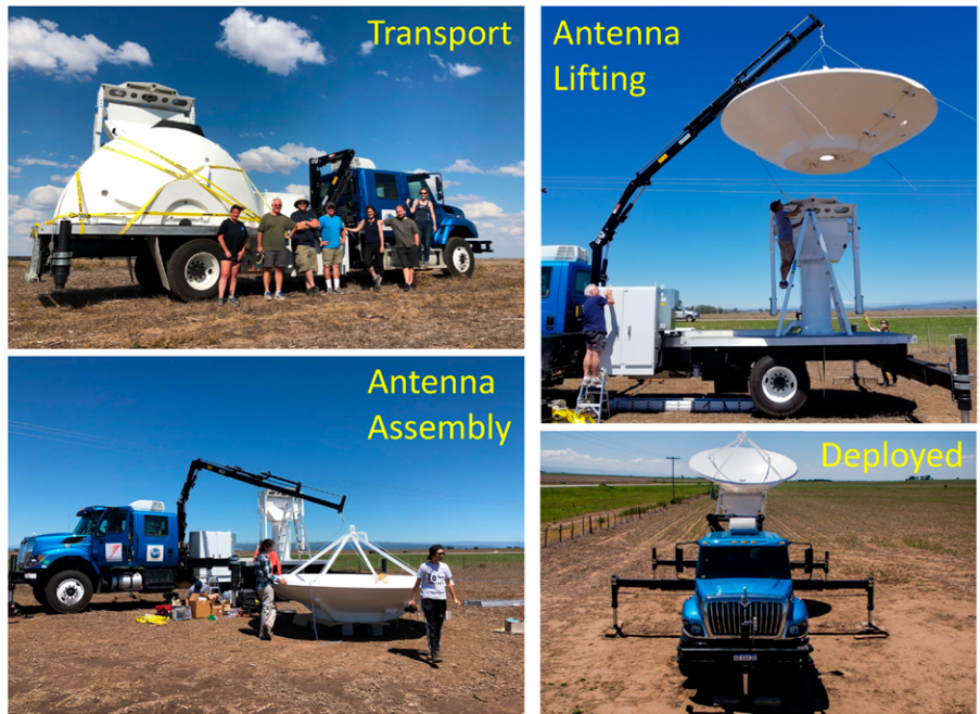
Fig. 8. COW assembly. COW as transported, antenna being assembled, antenna lifted onto pedestal, deployed.
