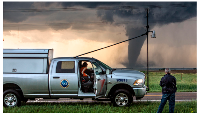
Fig. 9. FARM mobile mesonets (MM).
