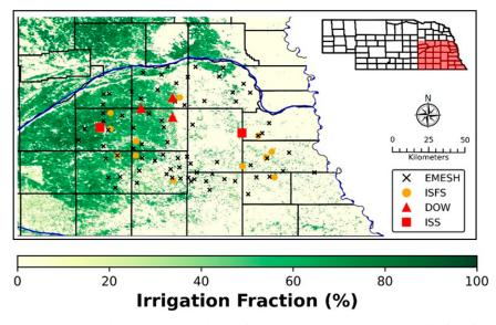
FIG. 1. Map of the GRAINEX study area in southeastern Nebraska. Data collection sites consisted of the 12 integrated surface flux system sites (ISFS), 2 integrated sounding system sites (ISS), 3 Doppler on Wheels deployment locations (DOW), and the 75 Environmental Monitoring, Economical Sensor Hubs (EMESH).
