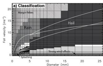
Parsivel Fallspeed-Diameter bins, typical fall speed curves for various hydrometeor categories and overlaid QC/hydrometeor category filtering regions. From Friedrich et al. (2014)
