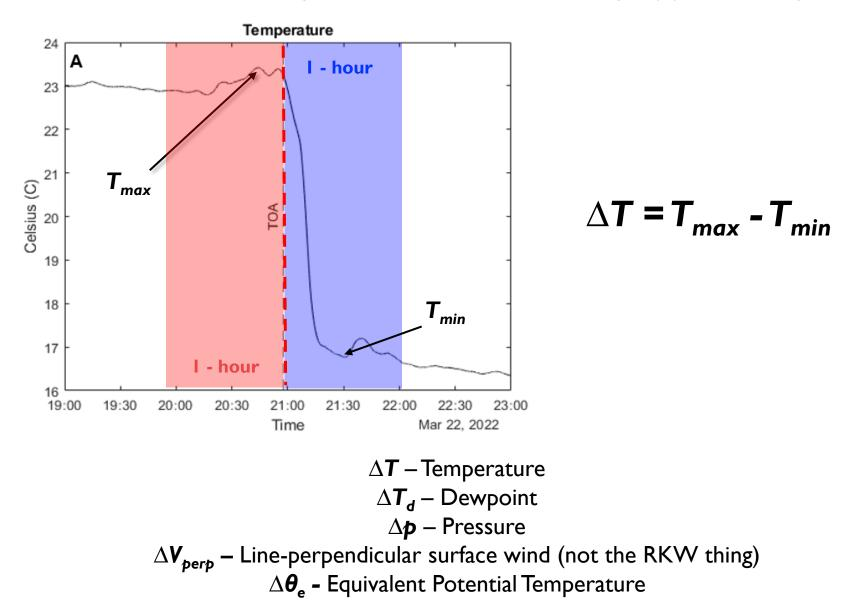
As the cold pool crosses the surface array, we can characterize each  $\Delta$  field at each instrument to capture spatial/temporal trends
