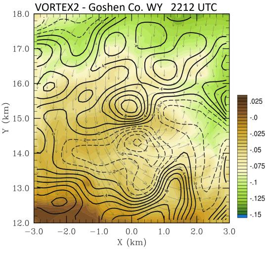
Terrain height in km relative to the altitude of the lowest radar (shaded); horizontal dual-Doppler wind (vectors); terrain-induced upward (solid) and downward (dashed) wind (W) contours.
