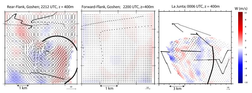
Difference between dual-Doppler horizontal (vectors) and vertical (shaded) velocity retrievals when solutions include/exclude objectively analyzed surface wind obs
