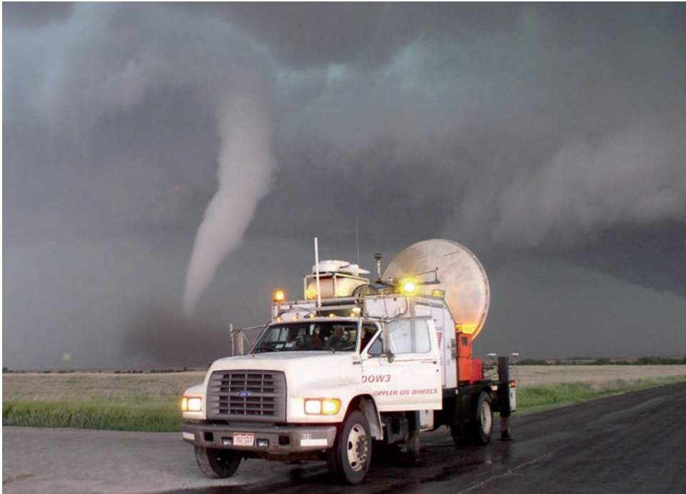
A Doppler on Wheels unit observing a tornado near Attica, Kansas. DOW radars scan through tornadoes and other small phenomena, collecting fine-scale 3D wind and reflectivity data
