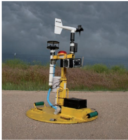
Pods weighing 50kg are dropped directly into the path of a tornado or along the coast for hurricanes at just 1m above ground level
