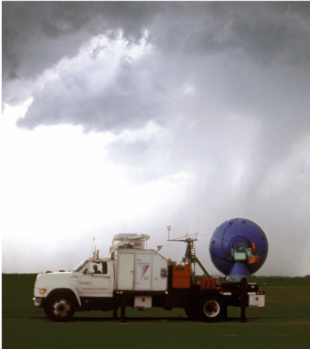
The Doppler On Wheels (DOW) project has created mobile weather radars mounted on trucks that explore rare, short-lived and small-scale phenomena
