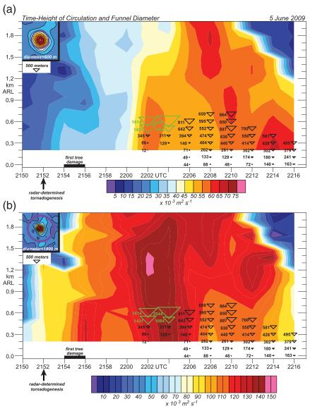
FIG. 7. Time-height plot of circulation ( $\times 10^3$  m<sup>2</sup> s<sup>-1</sup>) calculated from the dual-Doppler data over the area of a circle with diameter of (a) 600 and (b) 1800 m centered on the vertical vorticity maximum as shown in the inset diagrams. Superimposed numbers and symbols are as in Fig. 6.
