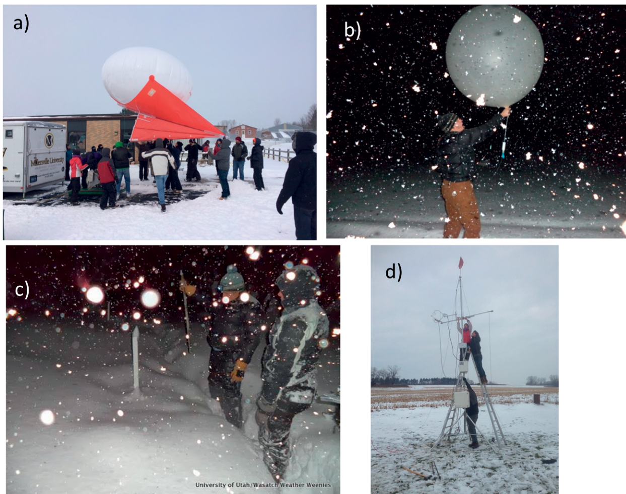
FIG. 8. Photos of students (a) launching a helium-filled kite (Helikite), (b) launching a radiosonde, (c) taking surface snow observations, and (d) servicing an instrumented tower during the OWLeS field operations. [Photos in (a),(d) were taken by R. Clark, MU, and those in (b),(c) by J. Steenburgh, UU.]
